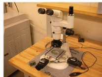
Digital microscope for full microscopic analysis of weld joint
